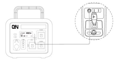
This product can be charged using the car charging port on the car. It needs to be charged after the car is ignited and started, so as not to cause the car battery to run out of power and fail to start. At the same time, make sure that the car charger port and the cigarette lighter of the car charger input line are in good contact. The company shall not be liable for losses caused by non-compliant operation.
